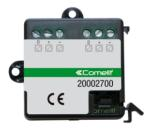
SimpleHome BUS separator/regenerator module. Enables you to isolate and regenerate the bus in systems with more than 40 modules. For direct connection to the SimpleHome BUS, creating islands with max. 40 modules. Possibility to separate only the BUS or also the power supply.
