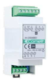
SimpleHome dimmer module for adjusting halogen and compact fluorescent (CFL) lamps, dimmable LEDs and electronic transformers. Power 300W. 1 input for connection of a control button. Dimmer function with control via a single or double button, motion detection function with energy saving which allows dimming of the lights when no movement is detected. DIN rail installation (2 modules). Dimensions: 35x90x58 mm. Max BUS absorption: 25 mA.
