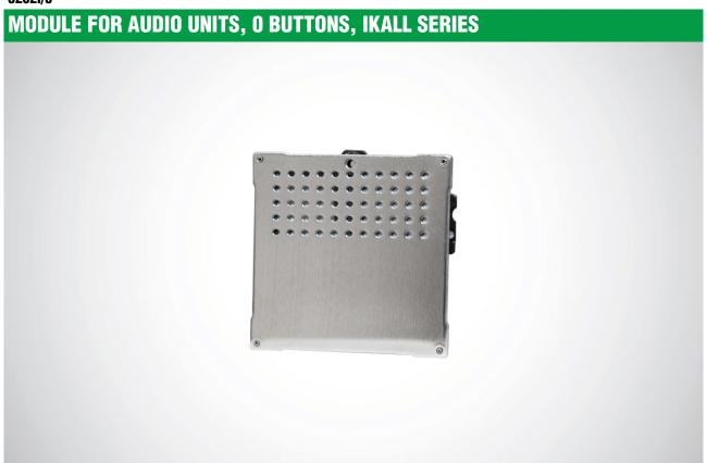
Made using double 2.5 mm stainless steel plate. To be equipped with an audio unit depending on the cabling system used. Fitted with a voltage reducer for powering festoon lamps if used with power supply unit 1595 or 1207. Dimensions 106x106x5.6 mm
