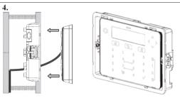
Connect the wiring and configure the keypad according to the supplied installation guidelines (refer to the Elegant Keypad Installer instructions). Insert the Elegant Keypad into the mounting bracket until it locks in place (see above).
