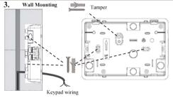
For walls (cement / breeze block), you can use the mounting template to measure the hole for mounting. Once the hole is opened, pull the keypad wiring through the knockout, insert the mounting bracket into the hole and secure with dibbles and screws (see above). Tamper can also be secured for tamper alarm activation (see above).
