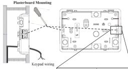
For room dividers (plasterboard), you can use the mounting template to measure a hole for mounting.
