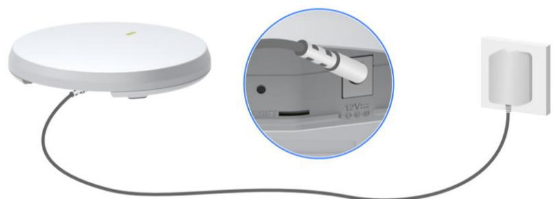
Figure 2-1 Connect Local Power Source
