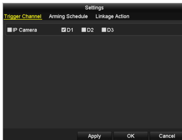
Figure 9-2 Set Trigger Camera of Motion Detection
