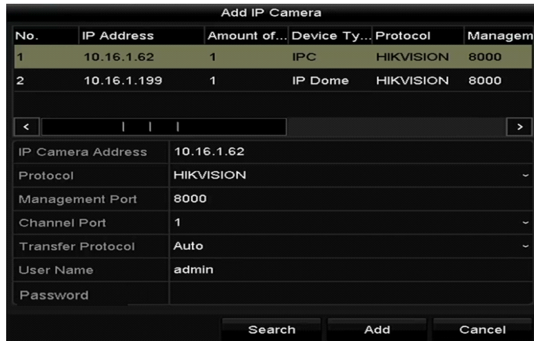
Figure 3-2 Quick Adding IP Camera Interface
