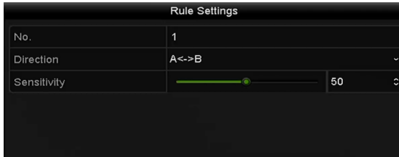
Figure 11-6 Set Line Crossing Detection Rules
