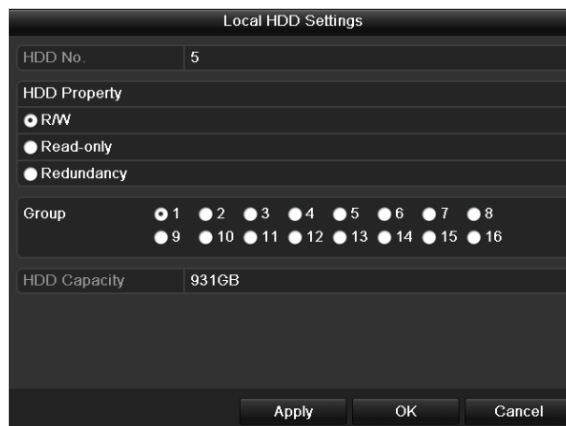
Figure 15-15 Local HDD Settings Interface
