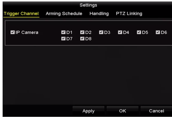
Figure 10-15 Set Trigger Cameras of POS
