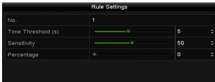
Figure 11-8 Set Intrusion Crossing Detection Rules
